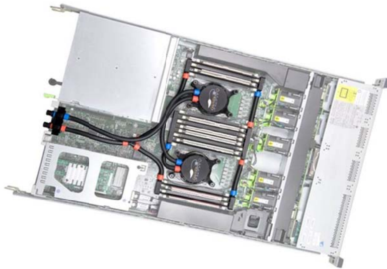
Figure 2.2.3.3 Liquid cooling system server Source: (Asetek Cooling Solution Company, 2020)
